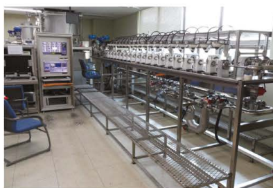
Water meter performance test corresponding to a given installation setup (15~50mm)
