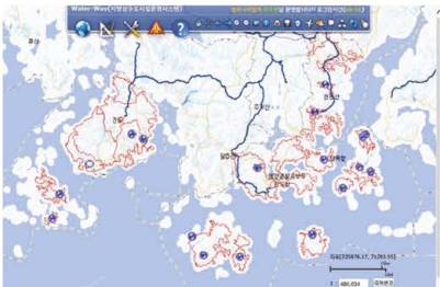
GIS-based management information on pipeline network and water supply facilities (workplaces and valves)
