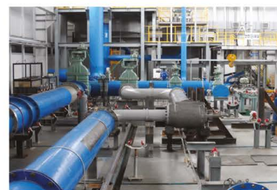
Precision control valve and fluid flow performance test (capacity factor, pressure recovery coefficient, and water hammer)
