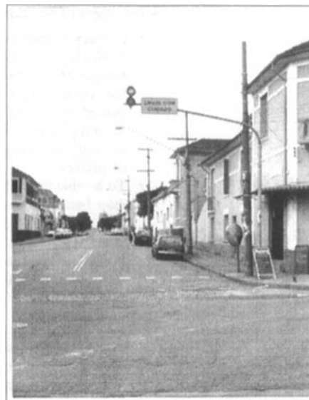
FIGURE 10.23 FLASHING YELLOW SIGNAL AND MESSAGE “PROCEED WITH CAUTION” ( CRUZE COM CUIDADO )
