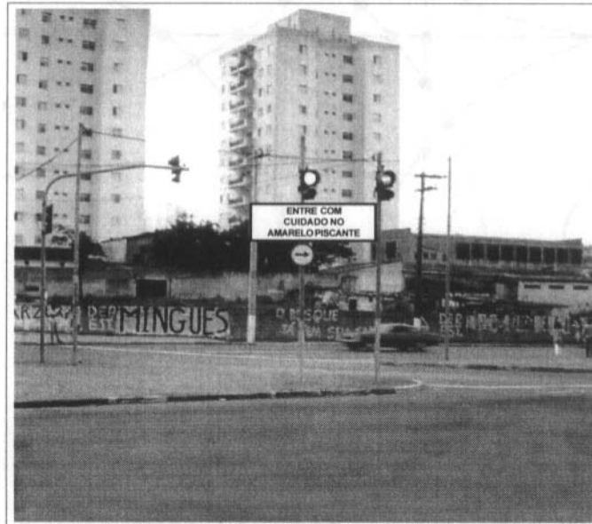
FIGURE 10.25 COMBINATION OF YELLOW FLASHING AND CONVENTIONAL SIGNALS ABRAÃO DE MORAES AVENUE x MIGUEL STÉFANO AVENUE (PROCEED WITH CAUTION ON FLASHING YELLOW - ENTRE COM CUIDADO NO AMARELO PISCANTE)
