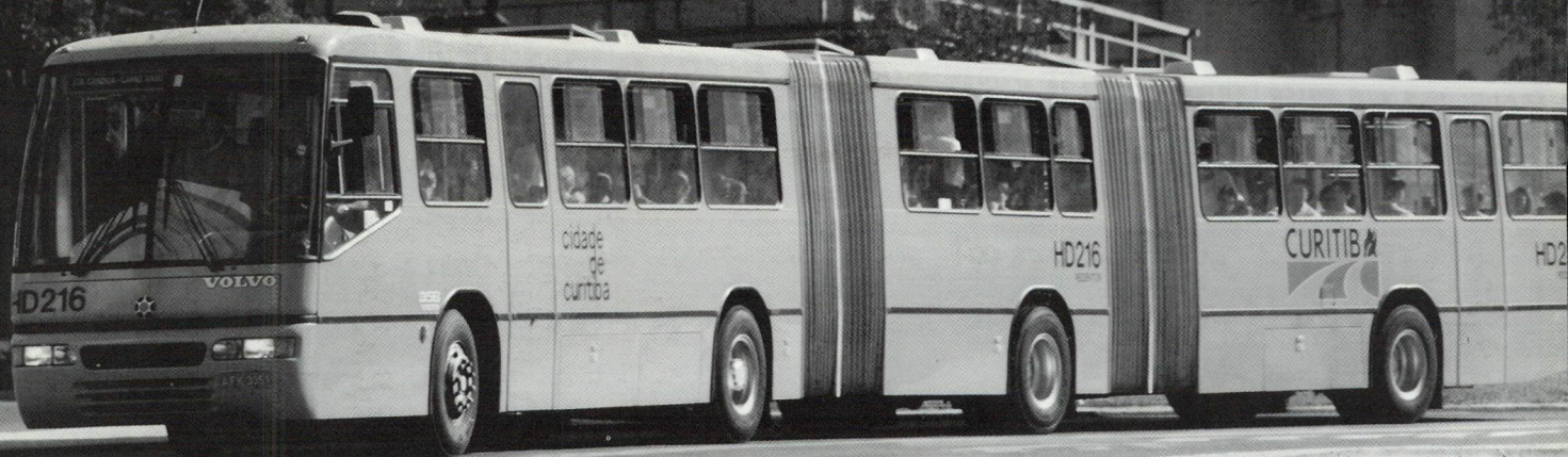
Two sides of Curitiba's transportation equation: its famous biarticulated buses and (below) well groomed bike paths. . .
