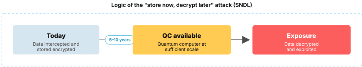
Figure 4. The “Store Now, Decrypt Later” (SNDL) attack flow: intercepting and storing encrypted data today to decrypt it once a sufficiently powerful quantum computer exists.
