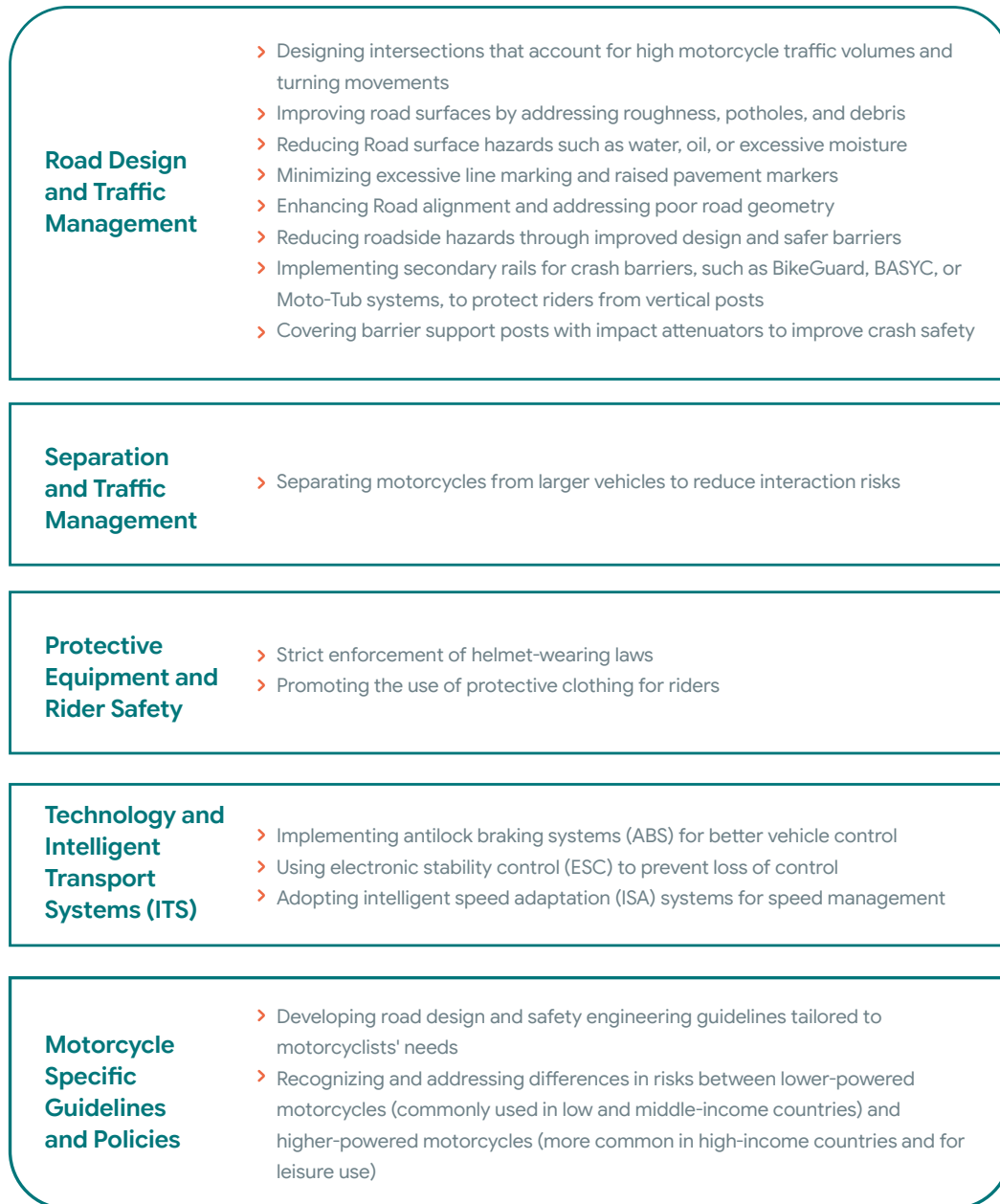
Figure 23. Key Measures and Specific Interventions for Improved PTW Safety Included in the iRAP Toolkit
