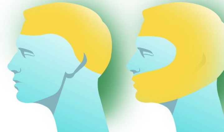
ILLUSTRATION 10 - PROTECTION AREAS IN HELMETS APPROVED UNDER UNECE R.22.05 STANDARD
