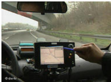
Figure1. GPS-based on board unit mounted on a truck (Source: http://www.tollroadsnews.com/cgi-bin/a.cgi/rwXBNI0REdmcEIJ61nsxIA )
