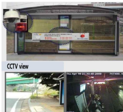
Figure 3 Crime prevention bell and CCTV
