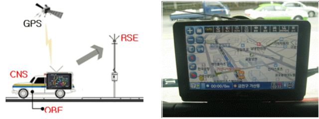
Figure 30 Communication between OBE and RSE (left) and OBE display
