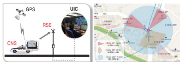
Figure 37 Road side equipment (left) and antenna range of various angles (right)
