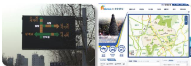
Figure 38 Variable message sign (left) and internet and mobile services (right)
