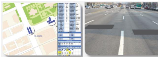
Figure 32 Cycle and signal management (left) and signal detector (right)
