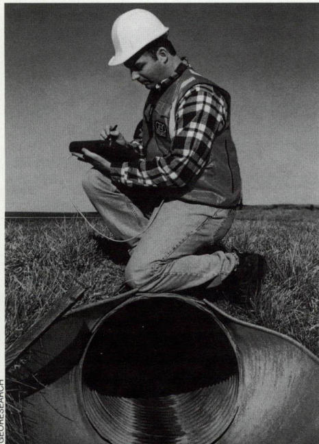
A technician armed with a GPS receiver records the location of a storm drain using a mapping system developed by GeoResearch, Inc. The system is used in many Latin countries to create precise digital maps and land-use databases.
