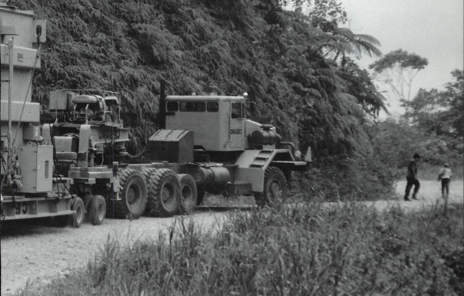
KING OF THE ROAD: A 60-wheel, 10-axle truck, moving at just 3 km per hour, takes five days to transport an 86-ton transformer from the Ucayali River to the Aguaytía power plant.
