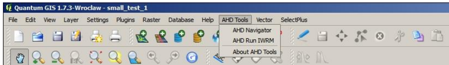
Figure A-4. AHD Tools menu. The AHD Navigator allows navigation on AHD flowlines and catchments.
