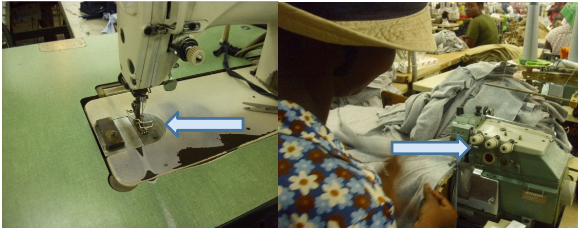
Figure 3. On the left is an example of a needle guard, also known as a finger guard, which protects against puncture injuries, while on the right is an example of an eye guard, which would shield the worker from any flying shards of needle if it should break. Note that the machine on the left is not equipped with an eye guard.
