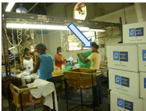
Figure 7. This illustrates the problem which is discussed in the preceding paragraph. The workers at this spot cleaning operation have been provided with loose-fitting dust masks (arrow), which are ineffective against chemical solvent vapors. However, it should also be noted that this location, with windows and overhead exhaust fan, may be preferable for these activities than the location in Figure 3.
