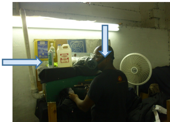
Figure 4. An example of a spot cleaning operation: the respirator is presumably the proper type; that depends upon the specific type of air-purifying cartridges which are provided (vertical arrow). Eye protection is provided, but note that gloves are missing. The ventilation at this work station is questionable: while there appears to be some type of local exhaust ventilation provided via the white pipe (horizontal arrow), the operation of the white fan on the right of the worker would likely disrupt any chance of its effectiveness, and appears to be positioned so that it will blow chemical vapors directly at the worker. Proper chemical selection, location and ventilation could eliminate the need for use of that respirator (imagine wearing it throughout the workday during the summer in Haiti).
