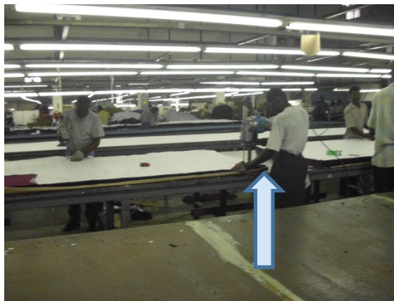
Figure 6. A cutting area in an apparel factory where workers are wearing metal mesh gloves while using blade knife cutters on sheets of fabric. The risk to their hands in the absence of such PPE is clear from the proximity of the hand to the moving blade (arrow).
