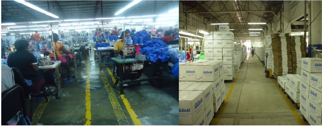
Figure 2. Examples of poor (on the left) and good (on the right) housekeeping and workplace organization, and how these factors may impact means of egress on the factory floor and the ability of workers to evacuate the building. Note on the left how the manufacturing equipment has been allowed to encroach upon the designated egress aisle.
