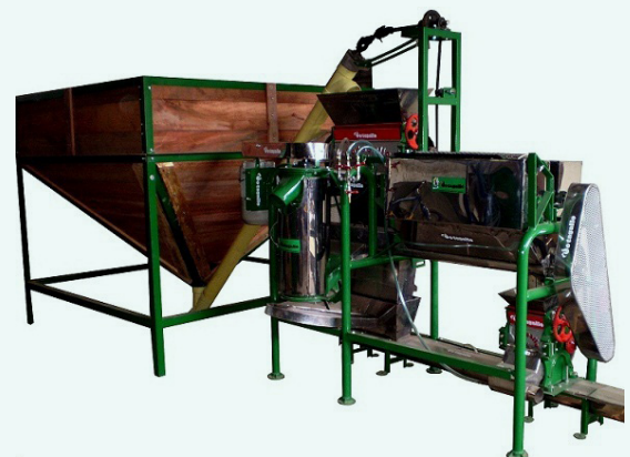
Ecomill machinery for producing parchment coffee. Inversiones Jotagallo S.A.
