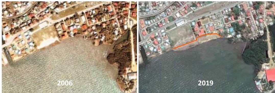
Figure 30. Reclaimed land on the eastern end of Belize City South PHS (orange line: 2006 shoreline).
