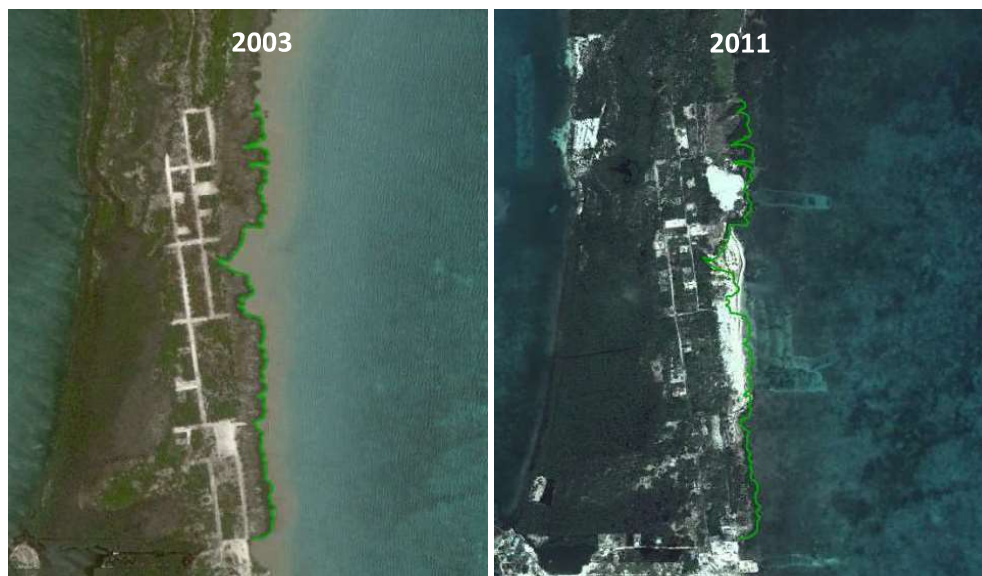
Figure 25. Removal of mangroves, beach nourishment and dredging of the seafloor on the central area of Caye Caulker North PHS (green line: 2003 shoreline covered with mangroves).
