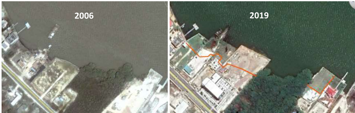
Figure 29. Reclaimed land on the western end of Belize City North PHS (orange line: 2006 shoreline).
