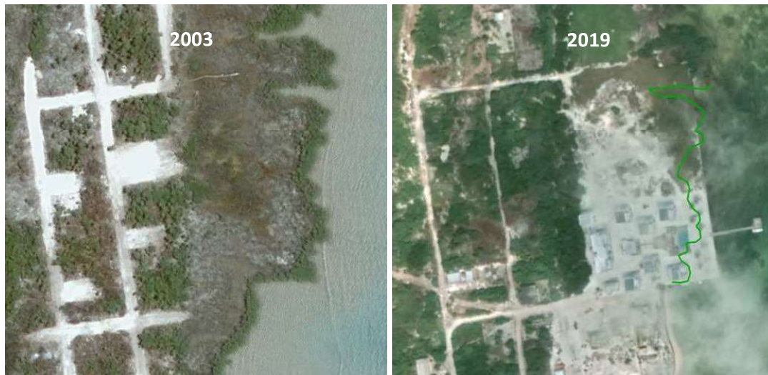
Figure 26. Removal of mangroves and land claim based on a seawall protection on the northern area of Caye Caulker North PHS (green line: 2003 shoreline covered with mangroves).
