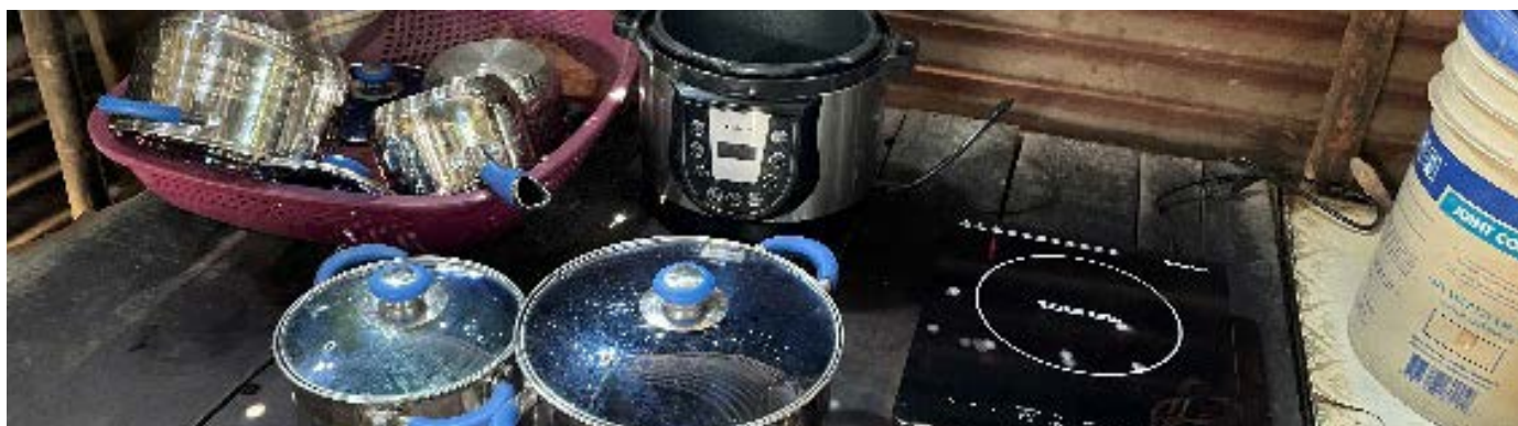
Technologies delivered: (i) induction cookstove with a set of pots and pans; and (ii) electric pressure cooker. Credit: Fundación Solar.
