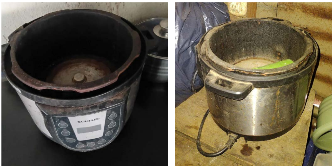
Electric pressure cookers damaged due to inadequate storage and hygiene practices in eleven households. Credit: Fundación Solar.
