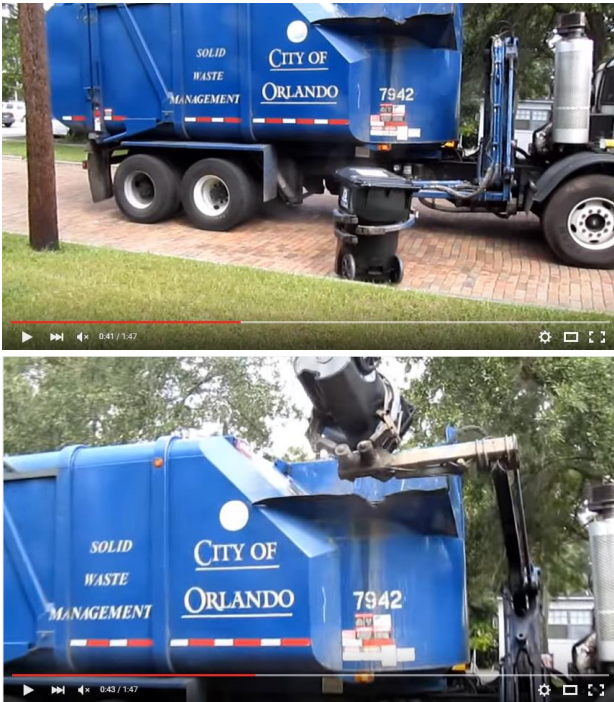
Figure 11 City of Orlando's automated garbage collection trucks (Source: FormerWMDriver, 2015)
